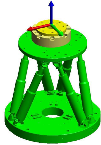
Figure 3 - Native hexapod co-ordinate frame in its CAD nominal position
