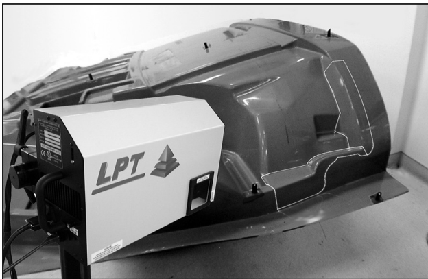
Fig. 3 - Laser Projection used to Indicate Composite Layout Position (Care of LPT)
