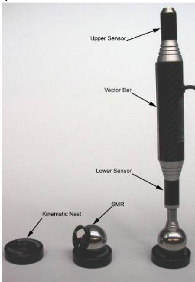
Figure 2 : Kinematic Nests with SMR and Vector Bar
