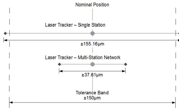
**Figure 6 - Experimentally determined uncertainty ( $\pm 3\sigma$ ) over a max distance of 14.5m in an uncontrolled environment; illustrating the benefit of using multi-lateration to reduce the impact uncertainty has on a tolerance budget.**
