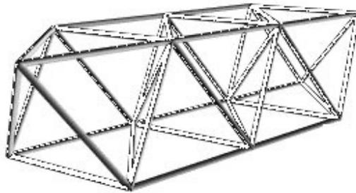
*Figure 5 - Tessellating arrangement of tetrahedral and octahedral elements*
