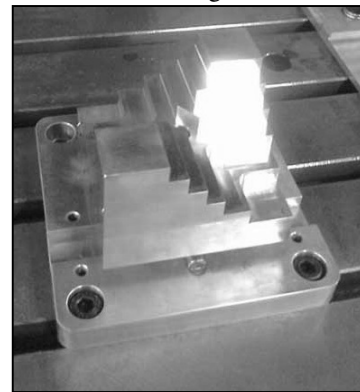
Fig.6: Initial Artefact used for 3-Axis Probing
